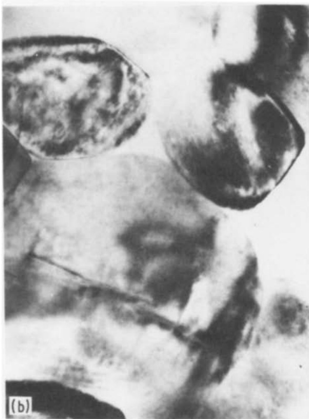
Figure 3 (a) Unmilled, sintered \text{ZrO}_2 (+2.3 mol % \text{Y}_2\text{O}_3 ) material (arrow points to crack); (b) milled, sintered \text{ZrO}_2 (+2.3 mol % \text{Y}_2\text{O}_3 ). Both (a) and (b) show light- and dark-field images to show the presence of glass.
